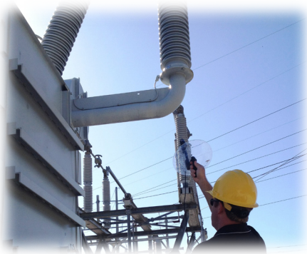
Parabolic sensor for corona effect detection
